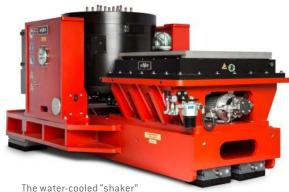
The water-cooled "shaker" used in our test lab
