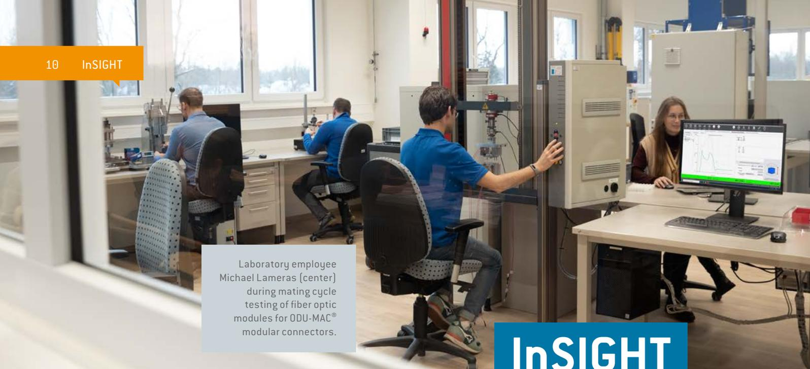
Laboratory employee Michael Lamas (center) during mating cycle testing of fiber optic modules for ODU-MAC<sup>®</sup> modular connectors.
