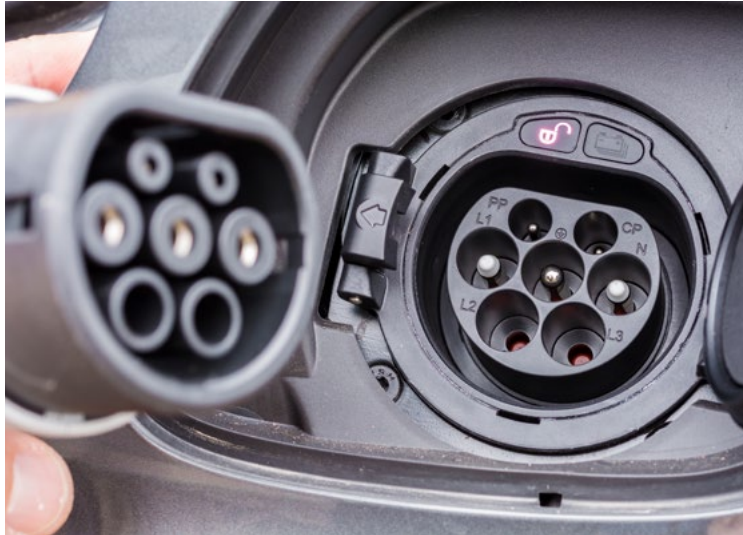
Fig 8. Type 2 plug & socket
