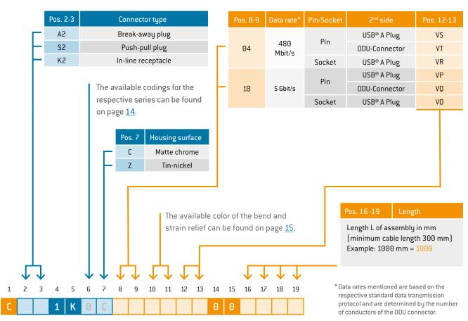
USB® without bend relief up to 1000 mm per single side assembly
