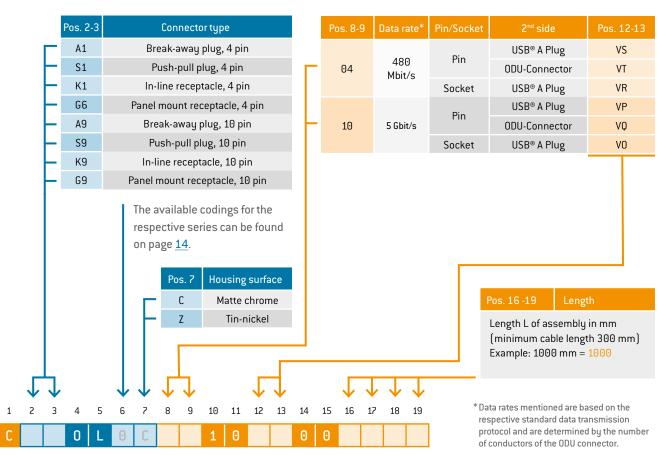
USB° with bend relief up to 3000 mm per single side assembly with transfer of 480 Mbit/s USB° with bend relief up to 2000 mm per single side assembly with transfer of 5 Gbit/s
