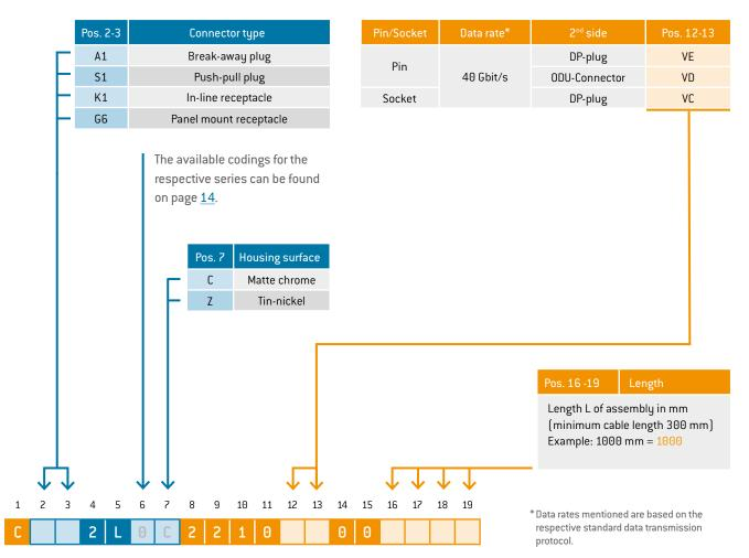
DisplayPort® with bend relief up to 4800 mm per single side assembly
