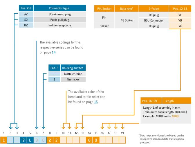
DisplayPort® without bend relief up to 4800 mm per single side assembly
