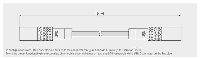
Pos. 2-3 Connector type USB® C Plug SA Push-pull plug ۷N Pin KA 10 Gbit/s In-line receptacle **ODU-Connector** ۷M GB Panel mount receptacle Socket USB® C Plug VLThe available codings for the respective series can be found on page <u>14</u>. Housing surface Pos. 7 Matte chrome Tin-nickel Length Length L of assembly in mm (minimum cable length 300 mm) Example: 1000 mm = 100012 15 18 10 11 13 14 16 19 \* Data rates mentioned are based on the
