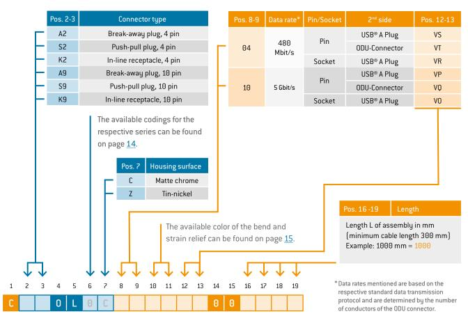
USB® without bend relief up to 1000 mm per single side assembly
