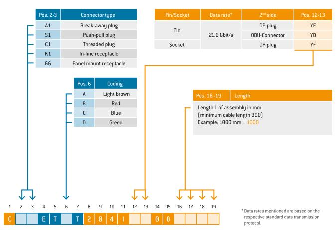
DisplayPort® without bend relief up to 4800 mm per single side assembly
