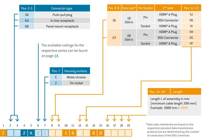
HDMI® with bend relief up to 3000 mm per single side assembly
