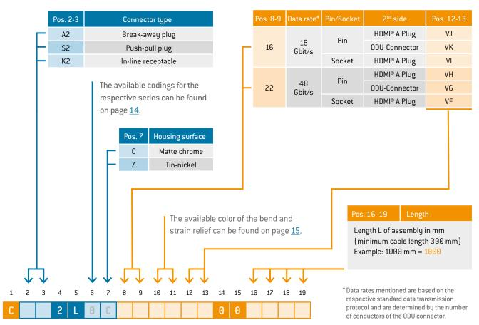
HDMI® without bend relief up to 3000 mm per single side assembly
