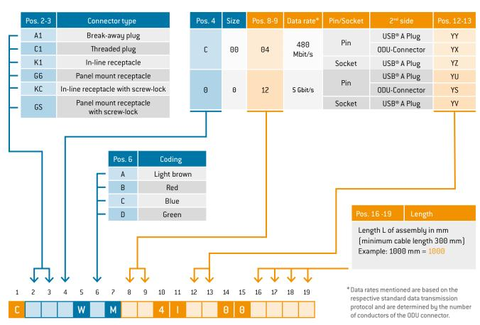
USB° without bend relief up to 3000 mm per single side assembly with transfer of 480 Mbit/s USB° without bend relief up to 2000 mm per single side assembly with transfer of 5 Gbit/s
