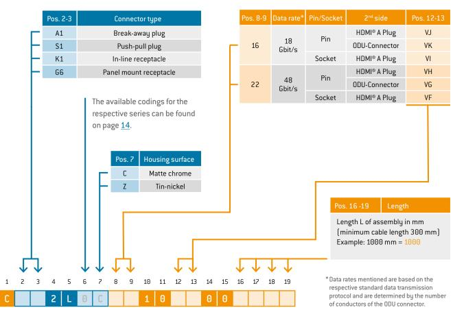
HDMI® with bend relief up to 3000 mm per single side assembly
