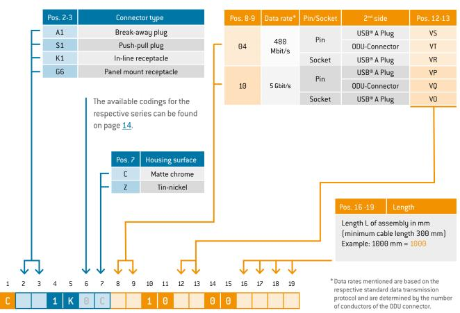
USB° with bend relief up to 3000 mm per single side assembly with transfer of 480 Mbit/s USB° with bend relief up to 2000 mm per single side assembly with transfer of 5 Gbit/s
