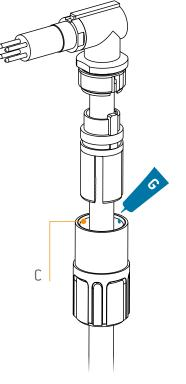
▶ Slide the assembled cable considering the guidings (B) into the housing. Slide the cable collet into the right-angled part and screw it with the back nut (C).
