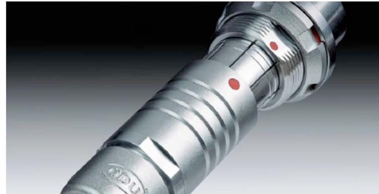
The ODU MINI-SNAP® F Series is an ideal self-locking circular connector for a wide range of applications due to its robust metal housing and wide range of sizes. Push-Pull locking mechanism for easy and secure mating and demating. IP50 protection - up to IP68 on select plug and receptacle housings, up to 5,000 mating cycles, 2-27 contacts and mixed configurations possible with 3 half shell coding options. The ODU MINI-SNAP® F Series can be terminated in solder, crimp and PCB.
