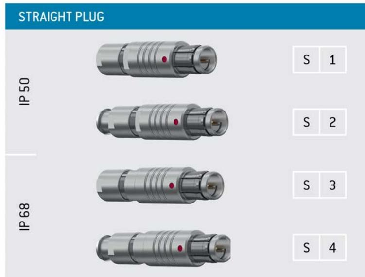
The Style S1/S2 and S3/S4 shown here are the two most commonly used straight plug housing styles. Housings styles S1 and S2 are IP 50 protected where styles S3 and S4 are IP68 protected in mated condition.
