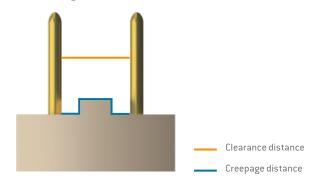
If these clearance distances collapse due to an excessively high field strength, electric flash-arcs occur. Flash-arcs do not only damage individual components such as connectors, but also endanger the well-being of patients and operators and may cause for example burns, muscle paralysis, right up to cardiac arrest.
